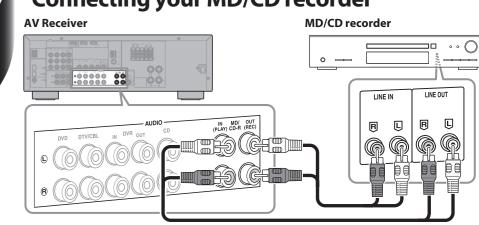
Use audio pin cables (not included) to connect your MD/CD player to the AV Receiver's MD/CD-R IN/OUT jacks, as shown.
