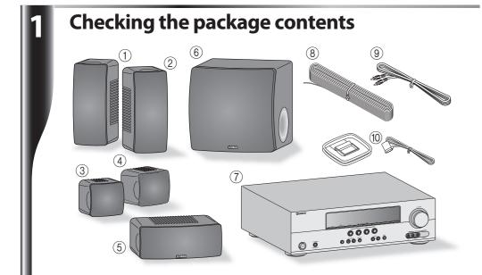
Unpack and check the package contents. The following items are necessary to complete this Connection Guide. See the owner's manuals for a complete list of supplied items.
