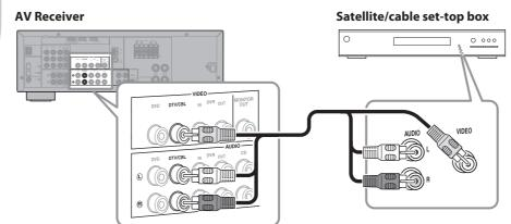
Use an AV pin cable (not included) to connect your satellite/cable set-top box to the AV Receiver's DTV/CBL jacks, as shown.
