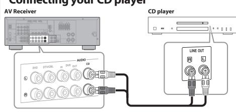
Use an audio pin cable (not included) to connect your CD player to the AV Receiver's CD jacks, as shown.
