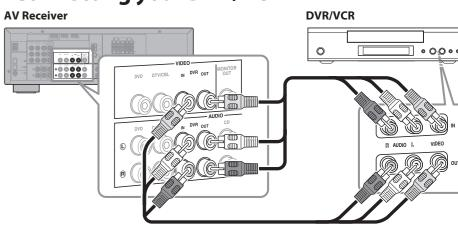
Use AV pin cables (not included) to connect your DVR (digital video recorder) or VCR to the AV Receiver's DVR IN/OUT jacks, as shown.
