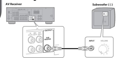
Use the included subwoofer cable to connect the Subwoofer's INPUT jack to the AV Receiver's SUBWOOFER OUTPUT jack.
