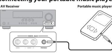
Use a 3.5 mm stereo mini plug cable (not included) to connect your portable music player to the AV Receiver's PORTABLE jack (on the front panel), as shown.
