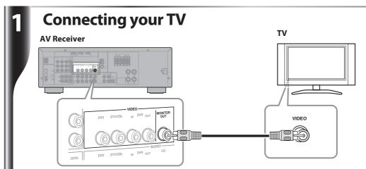
Use a video pin cable (not included) to connect the AV Receiver's MONITOR OUT jack to a composite video input on your TV, as shown.
