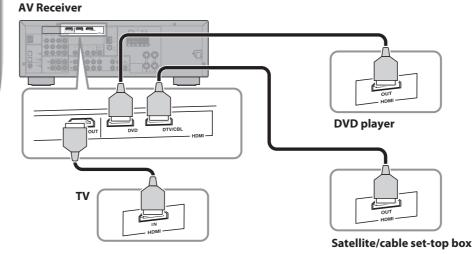
If your TV and DVD player or satellite/cable set-top box have HDMI jacks, you can connect them via the AV Receiver. Using HDMI cables (not included), connect the AV Receiver's HDMI OUT jack to an HDMI input on your TV, and connect your DVD player and satellite/cable set-top box to the AV Receiver's DVD and DTV/CBL HDMI jacks, respectively, as shown.
