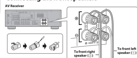
Connect the front speaker (1+2) cables to the AV Receiver. Be sure to connect the colored wire to the red positive (+) terminal, and connect the other wire to the black negative (-) terminal.
