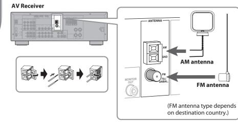
Connect the AM loop antenna and indoor FM antenna to the AV Receiver, as shown. See the owner's manuals for more information about connecting antennas.
