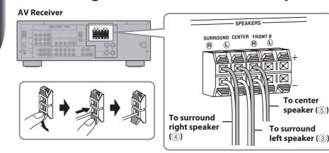
Connect the center speaker ( $\S$ ) and surround speaker ( $\S$ ) cables to the AV Receiver. Be sure to connect the colored wire to the red positive (+) terminal, and connect the other wire to the black negative (–) terminal.
