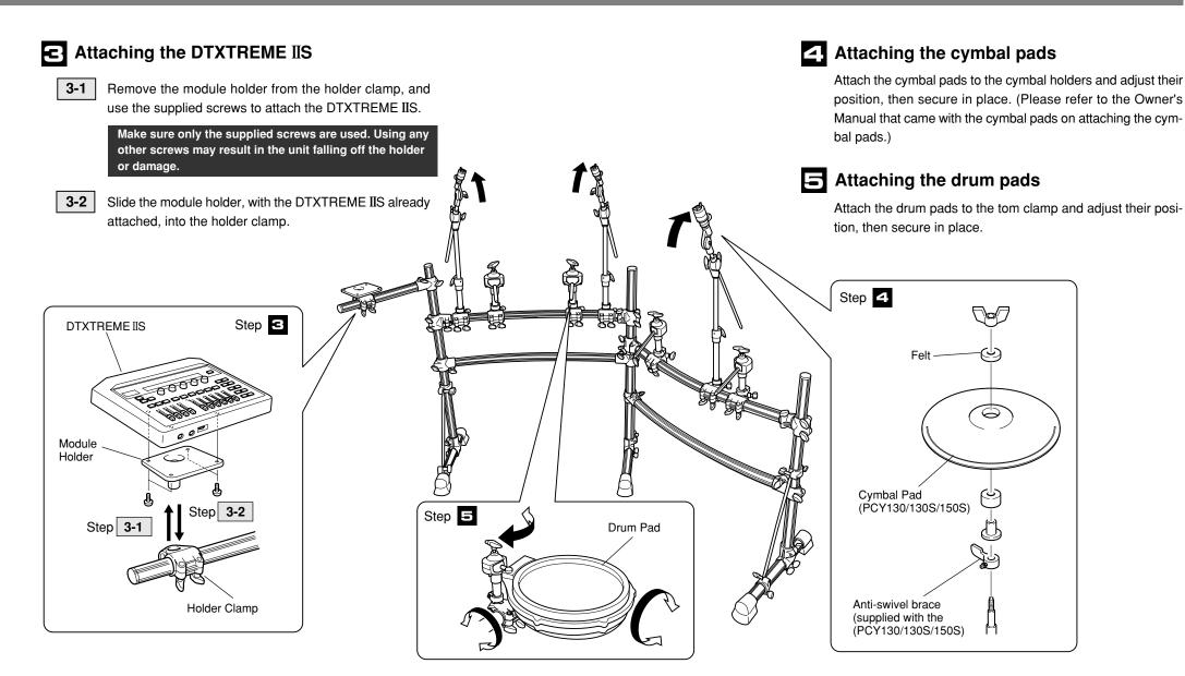
Maker sure all bolts on clamps, pads, etc., are tightened firmly.
