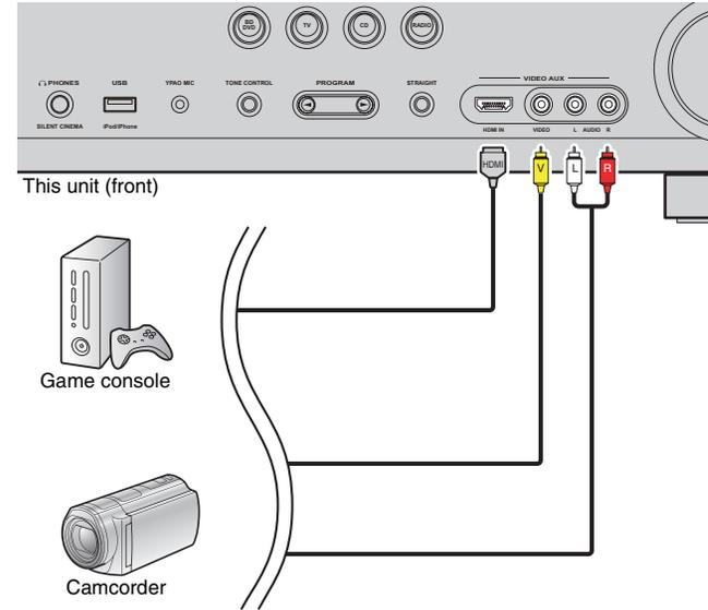
If you select "V-AUX" as the input source by pressing V-AUX, the video/audio played back on the device will be output from this unit.
