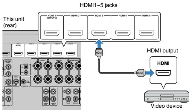
If you select the input source by pressing HDMI1~5, the video/audio played back on the video device will be output from this unit.
