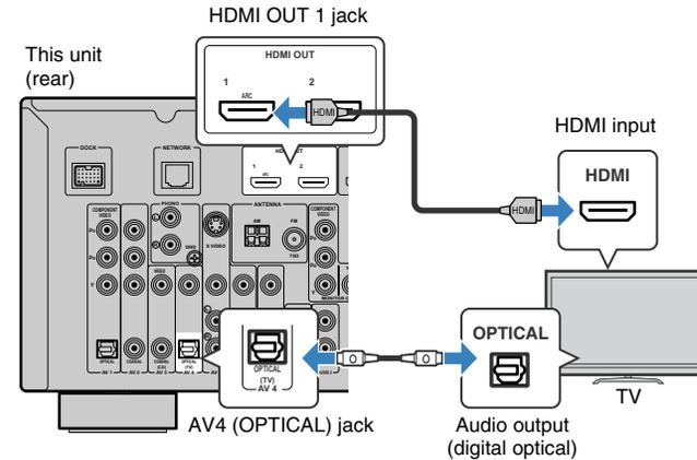
If switch the input source of this unit to "AV4" by pressing AV4 or SCENE(TV), the TV audio will be played back on this unit.
