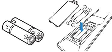
Insert into the remote control in the correct polarity (+/-)
