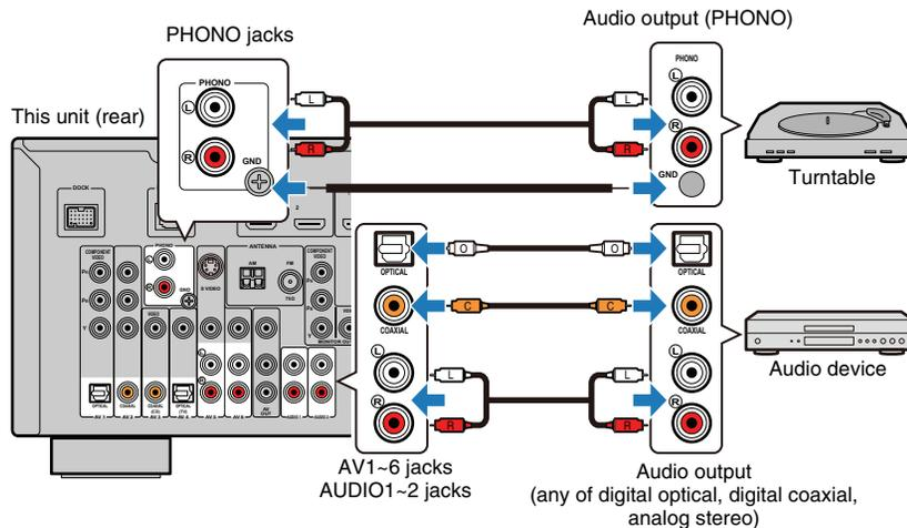
If you select the input source by pressing AV1~6, AUDIO1~2 or PHONO, the audio played back on the audio device will be output from this unit.
