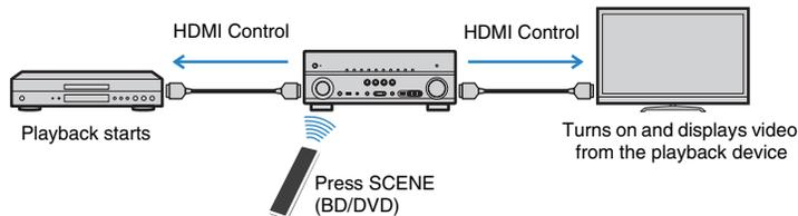
To use HDMI Control, you need to perform the following HDMI Control link setup after connecting the TV and playback devices.
