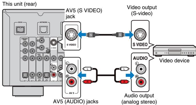
If you select the input source by pressing AV5, the video/audio played back on the video device will be output from this unit.
