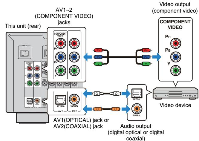
If you select the input source by pressing AV1~2, the video/audio played back on the video device will be output from this unit.
