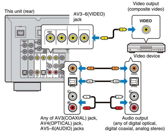
If you select the input source by pressing AV3~6, the video/audio played back on the video device will be output from this unit.
