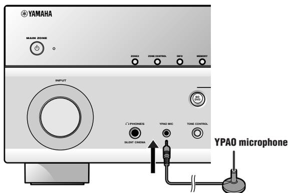
"Mic On. View ON SCREEN" appears on the front panel display, and then the display at right appears on the TV screen.
