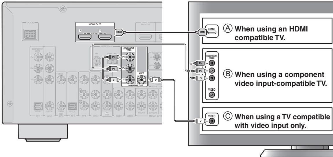
Video input to this unit is output to a TV using output jacks of the same kind.
