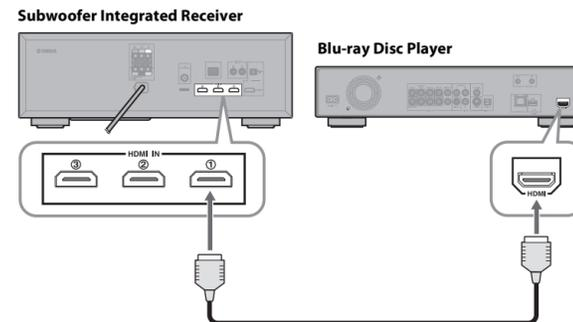
If your TV is HDMI-capable, you can connect it and Blu-ray Disc Player via the Subwoofer Integrated Receiver. Using the supplied HDMI cables, connect the Blu-ray Disc Player's HDMI output jack to the HDMI IN ① jack on the Subwoofer Integrated Receiver, as shown.
