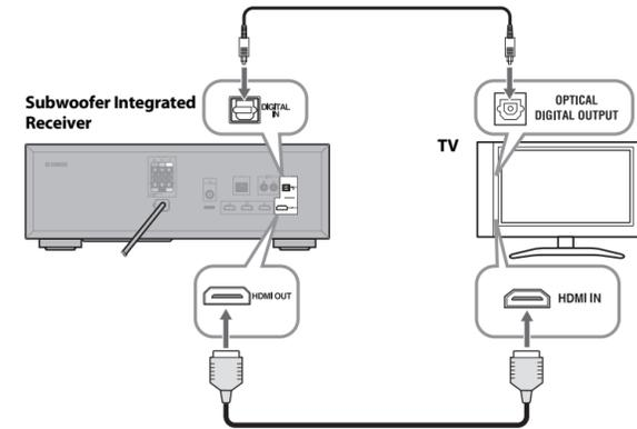
Connect your TV's HDMI jack to the HDMI OUT jack of the Subwoofer Integrated Receiver, using an additional HDMI cable, as shown.
