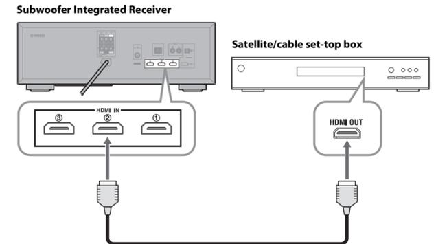
Use an additional HDMI cable to connect your satellite/cable set-top box to the Subwoofer Integrated Receiver's HDMI IN ② jack, as shown.
