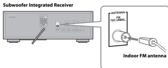
Connect the supplied indoor FM antenna to the Subwoofer Integrated Receiver, as shown. See the guides or manuals for more information about connecting an antenna.
