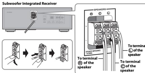
Connect the speaker cable to the Subwoofer Integrated Receiver. Be sure to insert the cable by matching the wire color with the color-coded terminal on the rear panel.
