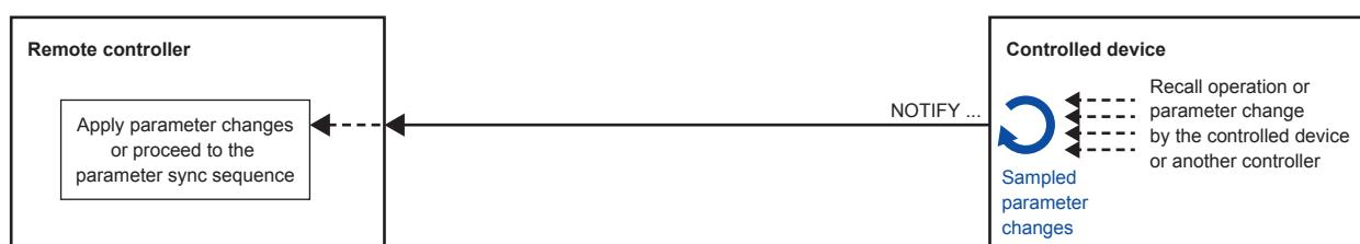
The way in which parameter change notifications are sent varies depending on the value notification mode specified in the MTX external control protocol mode.
