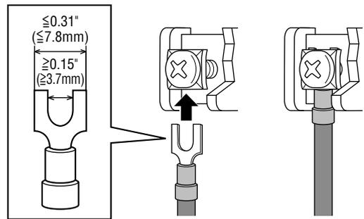
● **If using a bare conductor**
