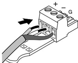
**3. Securely tighten terminal screws.**
