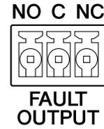
The [FAULT OUTPUT] connector (page 15) consists of NO (Normally Open), C (Common), and NC (Normally Closed) pins. The [FAULT OUTPUT] connector is a relay circuit that operates as follows.
