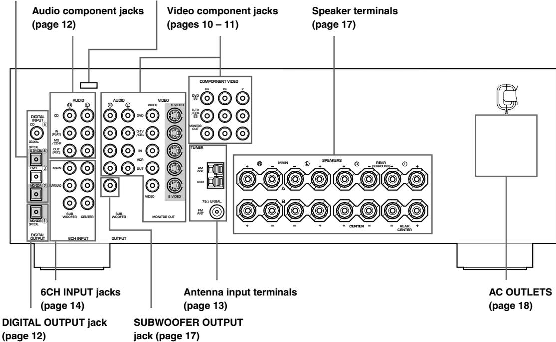
All illustrations of the rear panel in this manual are based on the RX-V540. The jacks in the shaded area in this illustration are not present on the RX-V440.
