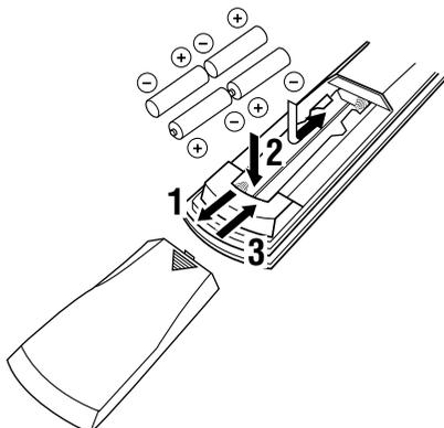
**1** Press the part marked with a ▼ and slide off the battery compartment cover.
