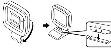
**2** Press and hold the tab to insert the AM loop antenna lead wires into the AM ANT and GND terminals.
