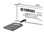
When the SD memory card has been correctly recognized, the [SD/ACT] indicator (page 9) will light. The [SD/ACT] indicator will flash while the card is being accessed.
