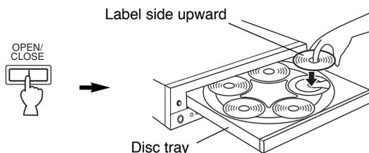
To play back an 8 cm (3 inch) CD, place it in the inner recessed area of the disc tray. Do not put a normal (12 cm (5 inch)) CD on top of an 8 cm CD.
