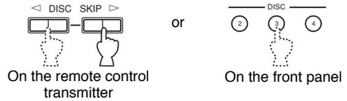
**5** Program a desired track by pressing the corresponding numeric button.
