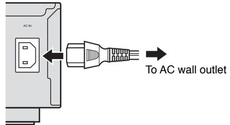
Plug the power cable into the AC IN, then plug the power cable to an AC wall outlet.
