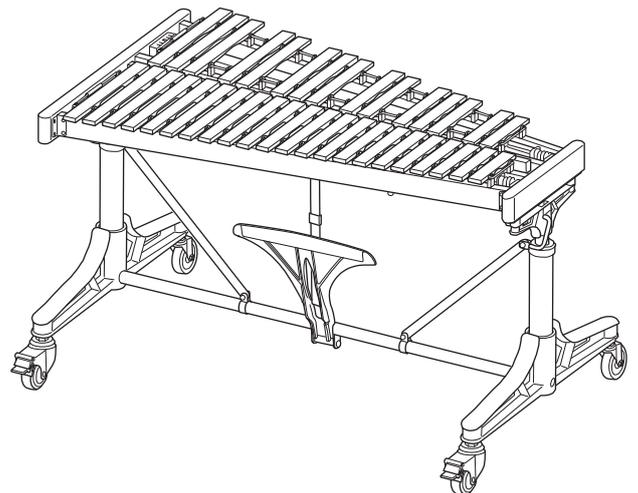
8. Lock the casters by pressing the stoppers of the left and right casters.
