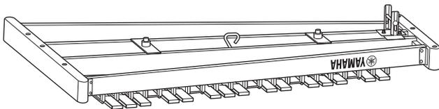
5. Turn the leg assembly upside down, put it on the main unit, and then secure it with the four screws.
