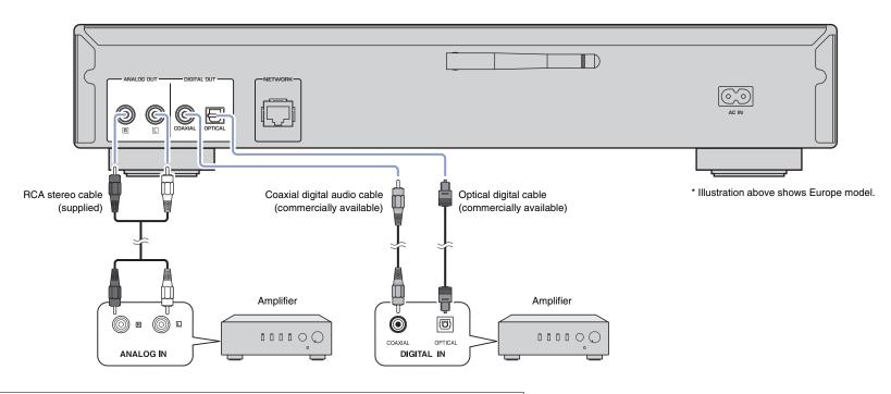
Only PCM signals can be output from the DIGITAL OUT (OPTICAL/COAXIAL) jacks of this unit.
