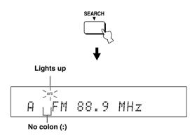
If a colon (:) appears in the front panel display, tuning is not available. Press PRESET/TUNE to turn the colon (:) off.
