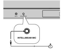
3 Place the IntelliBeam microphone on a flat level surface more than 1.8 m (6.0 ft) from the front of the unit and within 1 m (3.3 ft) upper or lower from the center height of the unit with the IntelliBeam microphone facing upward at your normal listening position.
