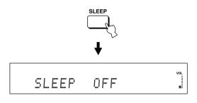
3 Wait for a few seconds without operating this unit to confirm the setting for the sleep timer. The SLEEP indicator disappears from the front panel display, indicating that the sleep timer is deactivated.
