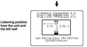
Select ANGLE TO WALL OR CORNER if this unit is installed in the corner of your listening room. Adjust the width and length of your listening room as well as the distance of the listening position from this unit.
