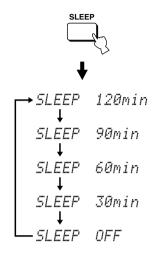
**3** Wait for a few seconds without operating this unit to confirm the setting for the sleep timer. The SLEEP indicator lights up in the front panel display, indicating that the sleep timer is activated.
