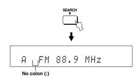
If a colon (:) appears in the front panel display, tuning is not available. Press PRESET/TUNE to turn the colon (:) off.
