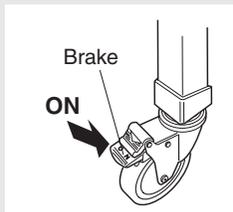
Playing the instrument without the brakes engaged can result in the instrument moving about or unwanted noise. Also, tuning or adjusting the pedal without the brakes engaged is very dangerous. The instrument can unexpectedly move or fall over resulting in injury.
