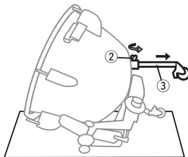
**4** Position the instrument as shown in the diagram below. Using both hands, turn the lock bolts **5** in the direction marked with the arrows until the narrow section of the lock bolt shaft **6** is visible.
