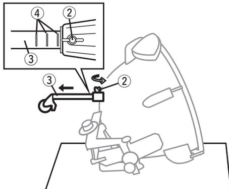
**3** Turn the instrument over and extend the other sliding leg using the same procedure.
