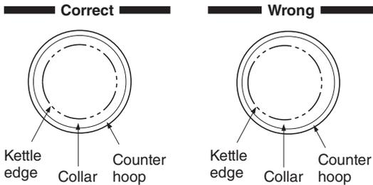
If collar width is not uniform, fully depress the heel end of the pedal. While holding the pedal in this position, realign the head and hoop as shown in the "Correct" illustration.
