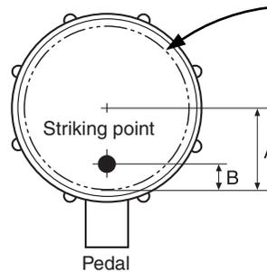
The standard striking point lies at distance B from the kettle edge, which corresponds approximately to 1/4 to 1/3 of the distance between the kettle edge and the center of the head.
