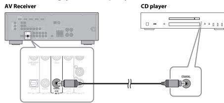
Use a digital coaxial cable (not included) to connect your CD player to the AV Receiver's AV 3 COAXIAL(CD) jack, as shown.
