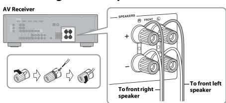
Connect the front speaker ((F)) cables to the AV Receiver. Make sure you connect the speakers with the correct polarity—positive (+) terminals to positive (+) terminals, and negative (-) terminals to negative (-) terminals.
