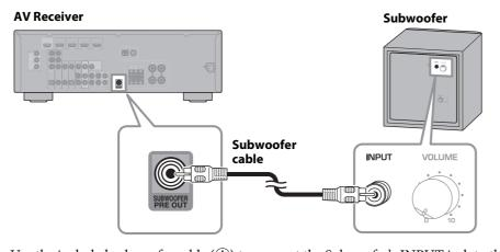
Use the included subwoofer cable  $(\begin{cal} \textcircled{1}\end{cal})$  to connect the Subwoofer's INPUT jack to the AV Receiver's SUBWOOFER PRE OUT jack.
