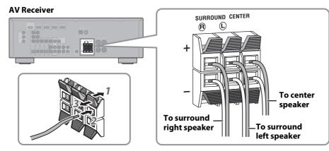
Connect the center speaker (G) and surround speaker (F) cables to the AV Receiver. Make sure you connect the speakers with the correct polarity—positive (+) terminals to positive (+) terminals, and negative (-) terminals to negative (-) terminals.
