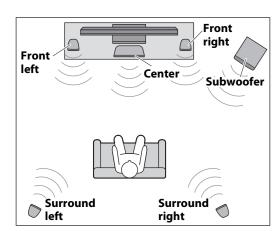
The four front and surround speakers are identical, so it doesn't matter which one you use in each position.
