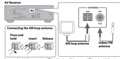
Connect the AM loop antenna  $(\bigcirc)$  and indoor FM antenna  $(\bigcirc)$  to the AV Receiver, as shown. See the owner's manuals for more information about connecting antennas.
