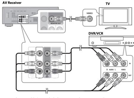
Use a video pin cable (not included) to connect the AV Receiver's MONITOR OUT jack to a composite video input on your TV, as shown.
