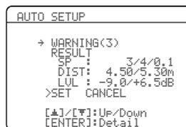
**2** Press **Ⓞ** / **◀** / **▶** repeatedly to toggle between the warning displays.
