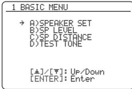
☀️ Set “TEST TONE” to “ON” to output the test tone for the “SPEAKER SET”, “SP LEVEL” and “SP DISTANCE”.
