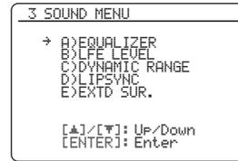
**5** Press **△ / ▽** repeatedly and then press **ENTER** to select and enter the desired submenu.
