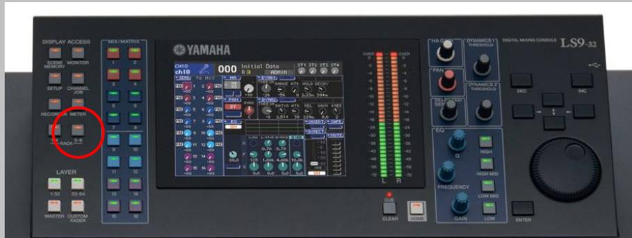
In the COMM PORT box, select “SLOT1” as the communication port for the MY16-ES64 card. (When using LS9-16, select “SLOT”.)
