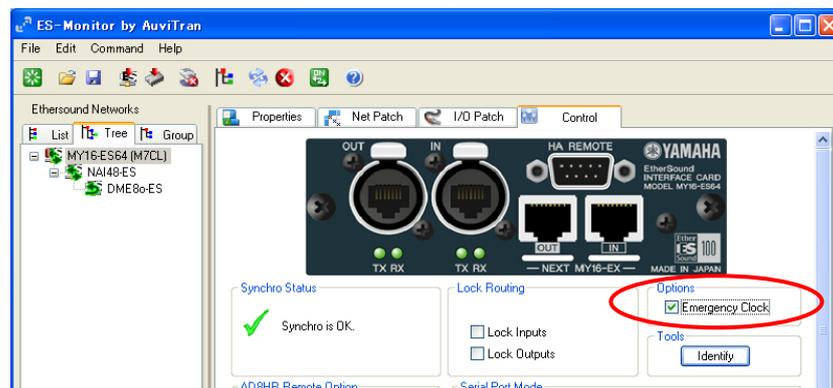
In the event of a cable failure, this clock is used during the interval until a new wordclock master is established.
