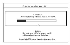
When installation is complete, the following message appears with the new firmware version. Press the power button on the instrument to turn it off and remove the USB memory from the instrument.
