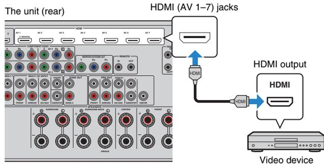
If you select the input source by pressing AV 1-7 on the remote control, the video/audio played back on the video device will be output from the unit.
