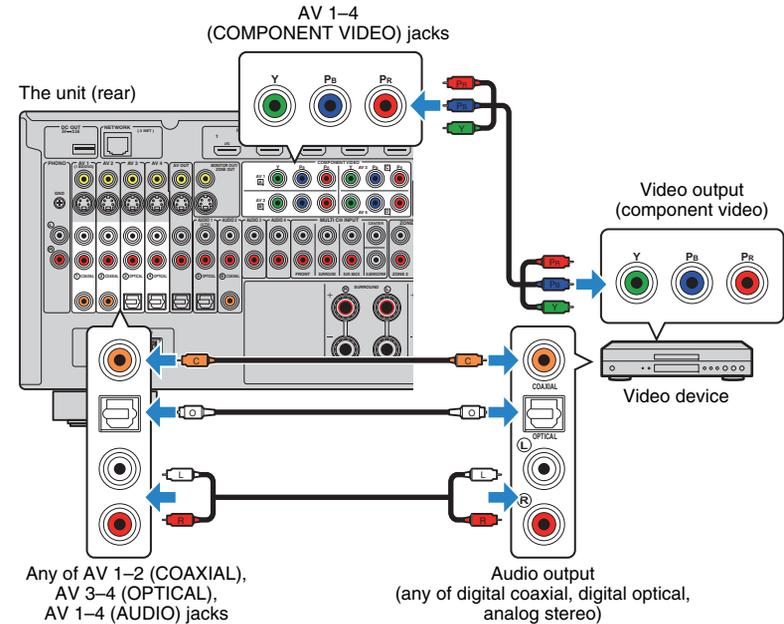
If you select the input source by pressing AV 1-4 on the remote control, the video/audio played back on the video device will be output from the unit.
