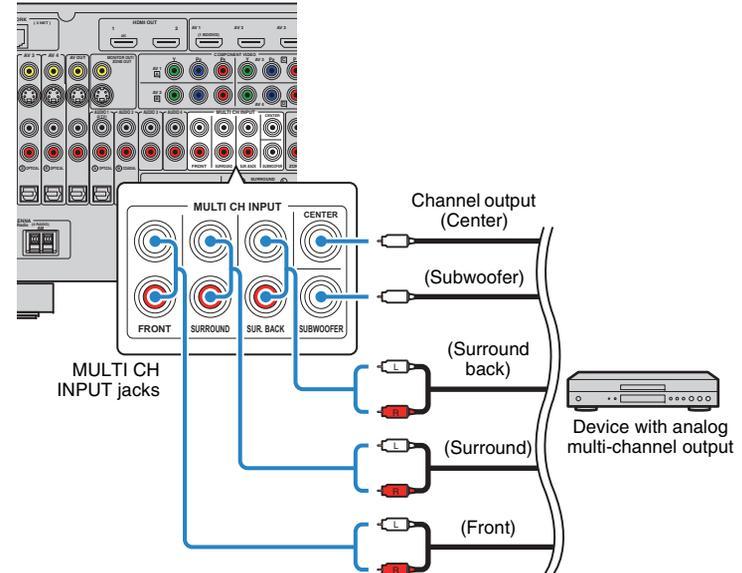
If you select "MULTI CH" as the input source by pressing MULTI on the remote control, the audio played back on the device will be output from the unit.
