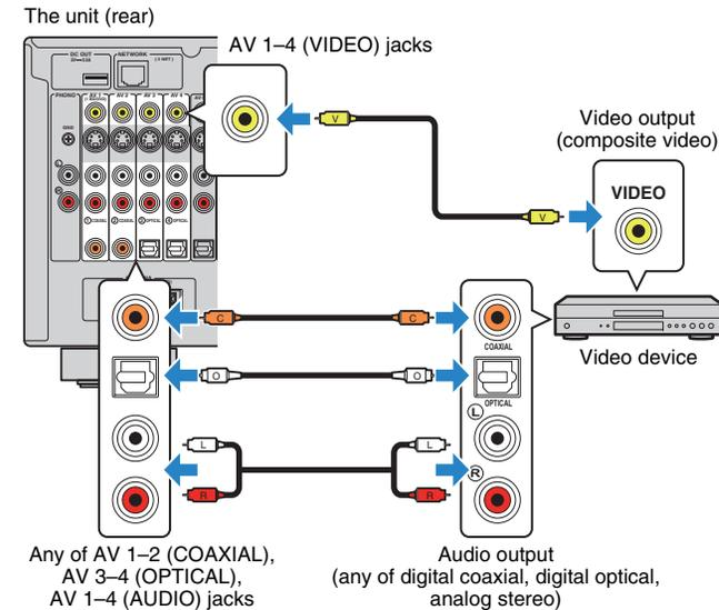
If you select the input source by pressing AV 1-4 on the remote control, the video/audio played back on the video device will be output from the unit.
