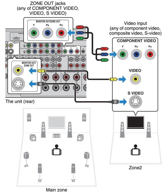
To assign the MONITOR OUT/ZONE OUT jacks to the Zone2 video monitor, set "Monitor Out Assign" (p.110) in the "Setup" menu to "Zone2".
