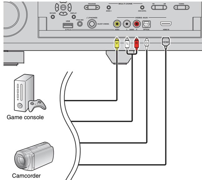
If you select "V-AUX" as the input source by pressing V-AUX on the remote control, the video/audio played back on the device will be output from the unit.
