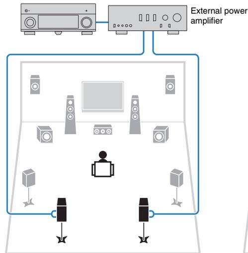
**Using the excess internal amplifiers for stereo speakers in another room**
