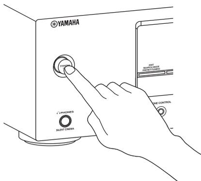
This unit is set to the standby mode. In the standby mode, this unit consumes a small amount of power in order to receive infrared signals from the remote control. To turn on this unit from the standby mode, press **(A)STANDBY/ON** (or **(B)POWER**). See page 21 for details.
