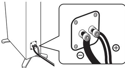
Cables are colored or shaped differently, perhaps with a stripe, groove or ridge. Connect the striped (grooved, etc.) cable to the “+” (red) terminals of your speaker. Connect the plain cable to the “-” (black) terminals.
