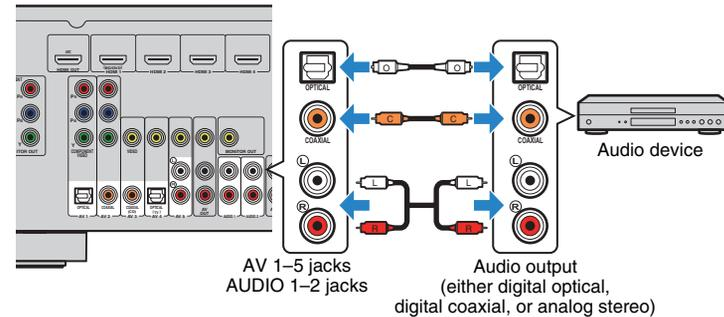
If you select the input source by pressing AV 1-5 or AUDIO 1-2, the audio played back on the audio device will be output from the unit.
