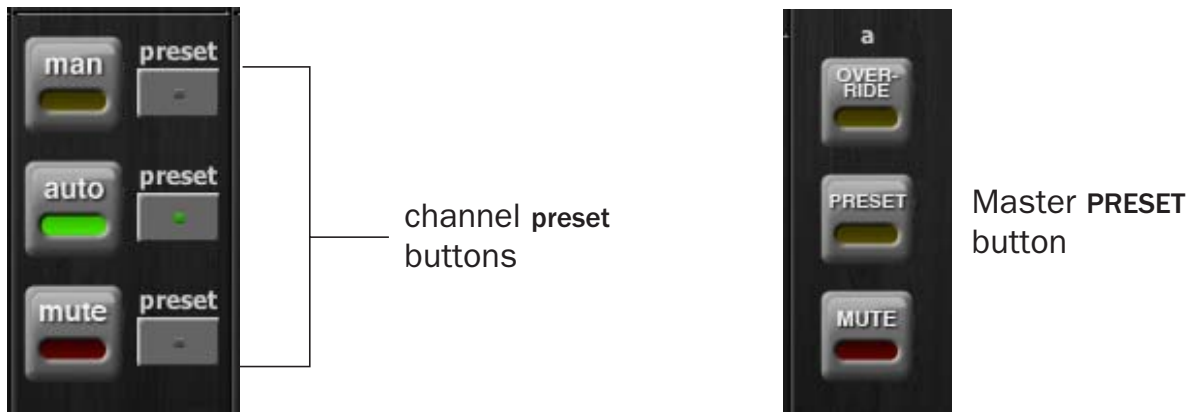
Figure 3-6 Channel preset (left) and Master PRESET (right) buttons
