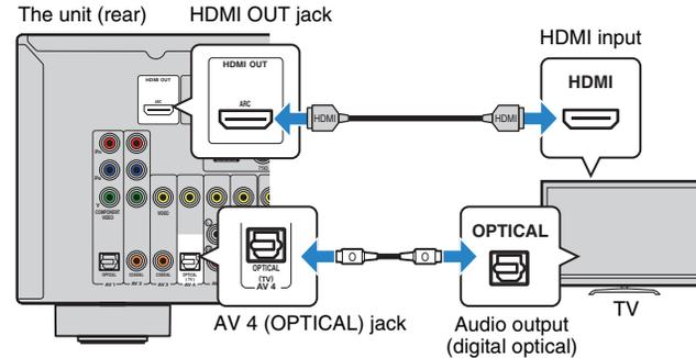
If you switch the input source of the unit to "AV 4" using the AV 4 or SCENE(TV) keys, the TV audio will be played back on the unit.
