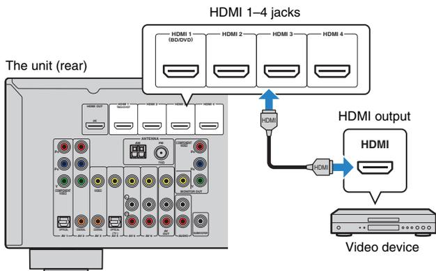
If you select the input source by pressing HDMI 1-4, the video/audio played back on the video device will be output from the unit.
