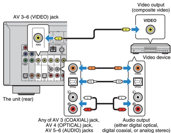
If you select the input source by pressing AV 3-6, the video/audio played back on the video device will be output from the unit.
