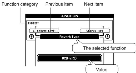
**4** Use the dial, the [+ ] and [- ] buttons, or the [0]–[9] number buttons to set the selected function as required.
