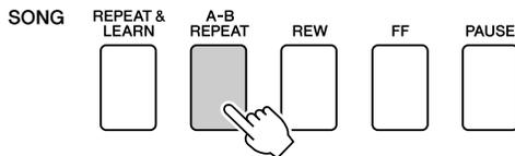
**2** Press the [A-B REPEAT] button a second time at the end of the section you want to repeat (the "B" point).
