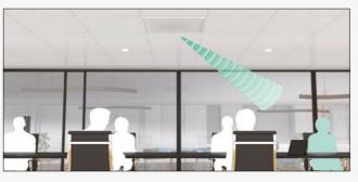
Multi-beam Tracking is a signal processing technology that can track multiple speaking participants by combining the use of beamforming technology to form directivity with multiple microphone elements to pick up sound. With multiple beams, each beam tracks different speakers' voices when multiple speakers are present.
