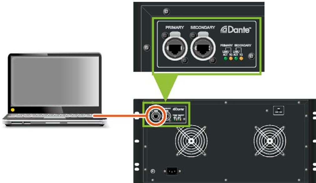
This figure is a connection example of the Rio3224-D.
